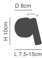
77-3517-23 SE-127-1AN LED, 1xE27, 3W, 230V
